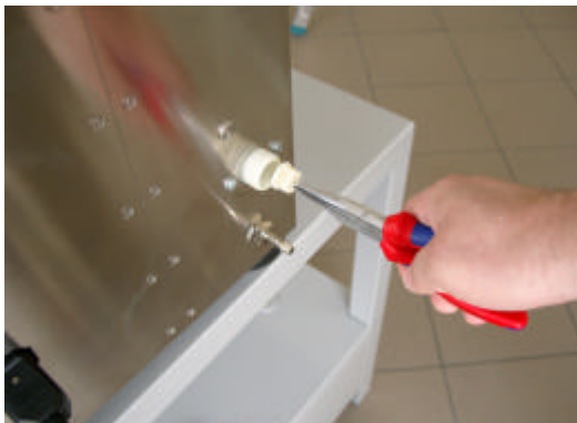
Illustration 4: Position of the water filter in the water inlet connection
